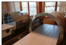
Figure 1: MITS 1.5/64 MHz (right) and 3.0/128 MHz (left) bench top exposure systems [2].
