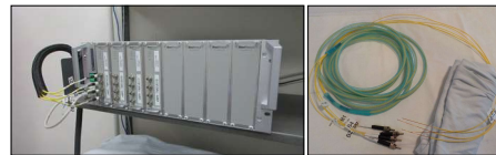
Figure 4: Omniflex temperature system (left) and T1C fiber optic temperature probes (right) [4].
